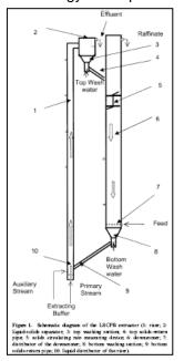
reactors - developed by the Universitv of Western Ontario (UWO) Department Chemical of and Biochemical Engineering. The continuous flow process could simultaneously adsorb and then release proteins using inter-connected two fluidized beds. The technology could be adapted for soy protein and protein sub-unit separation if researchers identified the riaht reactants and parameters. A new gentle process to separate protein inputs made from in Canada without the use of
