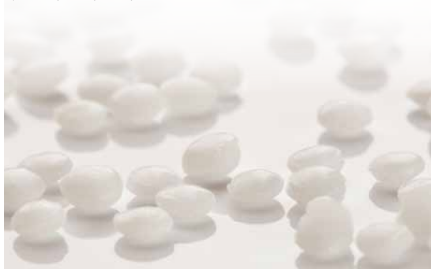
Soy wax pellets, used for candles and a variety of industrial and consumer applications.
